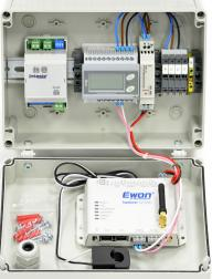
Typical HMS Networks/Uniq Solutions Ltd BEMS in a Box with Intesis Gateways
